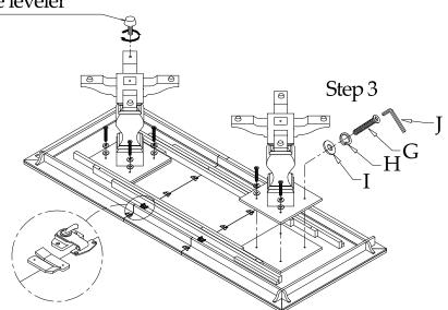
Step 3: With the Table Top placed upside down, position the assembled bases onto the bottom of the Table Top. Connect with the 1-3/8" Allen Head Bolts (G) and the same Washers as used in previous steps. Tighten with the Allen Wrench.
