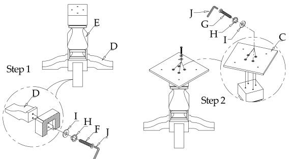
Step 1: Attach the Base Feet (D) at the bottom of the Pedestal (E) using the 3" Allen Head Bolts (F) Spring Washers (H) and Flat Washers (I). Tighten using the Allen Wrench (J).
